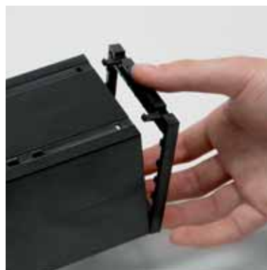
Fissare il circuito stampato montando la cornice posteriore Fix the printed circuit board by settling the rear frame
